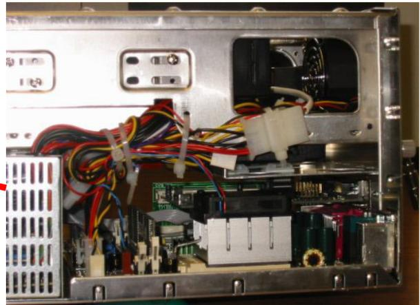
Figure 1.4 – Right hand side view internal showing mounting of M20 Terminal and custom power connector enclosure
