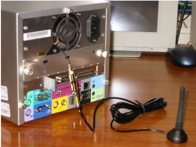
Figure 1.1 -Backplane of SV24 showing serial port expansion card and GSM terminal aerial connector with aerial
