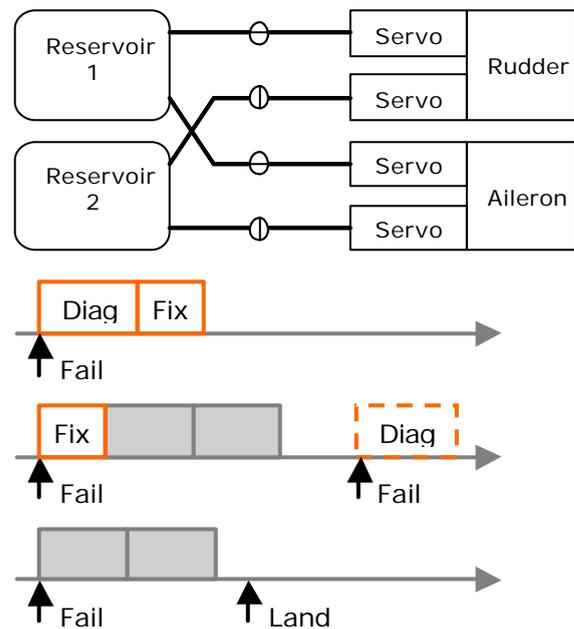
Fig. 1. Hydraulics system (top). Leaks can occur in the servos or reservoirs. Lower diagram shows scheduling options.
